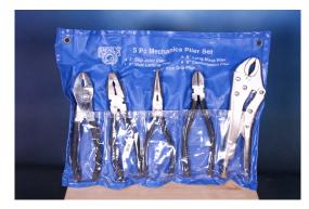
8" slip joint plier 8" side cutting plier 8" long nose plier 8" combination plier 10" vice grip plier
